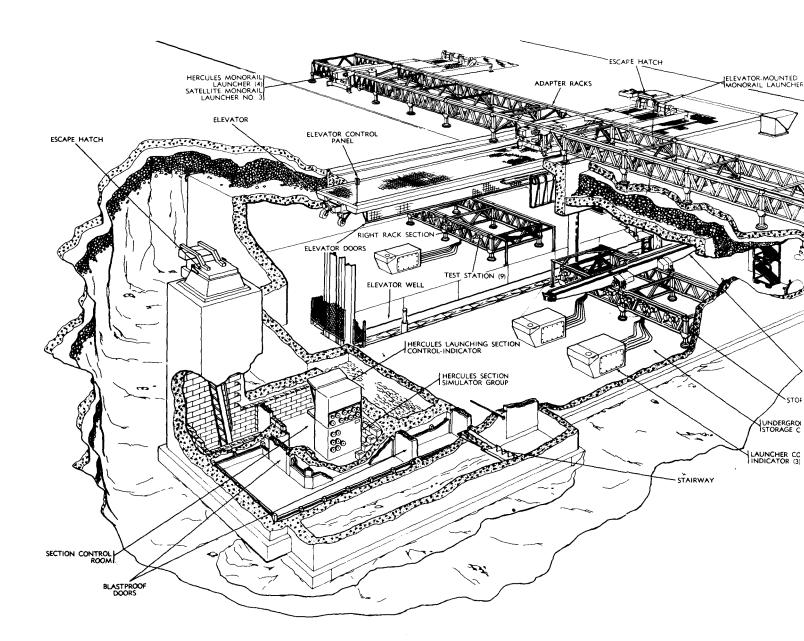
Figure 11. Launcher layout (permanent launching section
