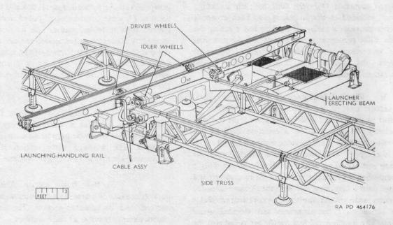
Figure 10. Hercules monorail launcher.
