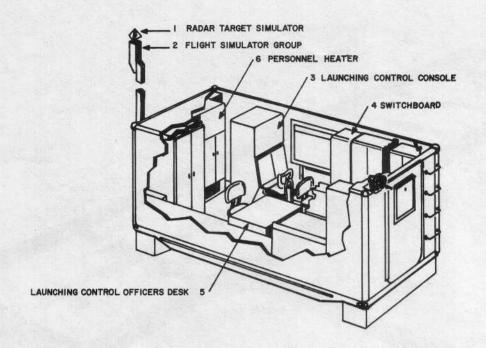
Figure 5. Launcher control trailer-permanent layout.
