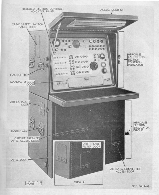
Figure 7. Launching section control indicator and section simulator group.
