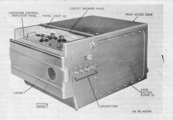
Figure 9. Launching control indicator.
