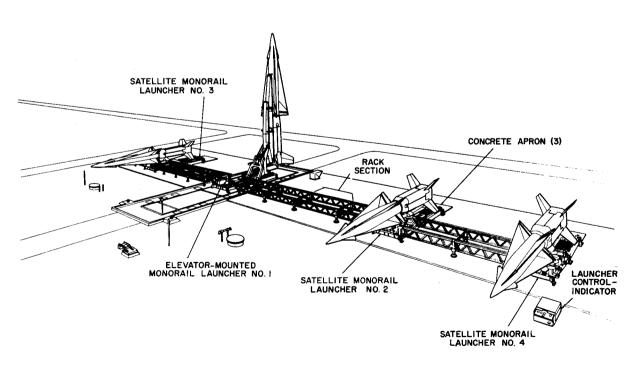
Figure 4. Nike Hercules launching section--permanent installation.
