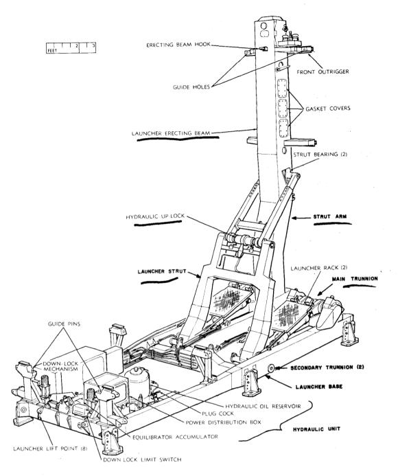
Figure 12. Monorail launcher.
