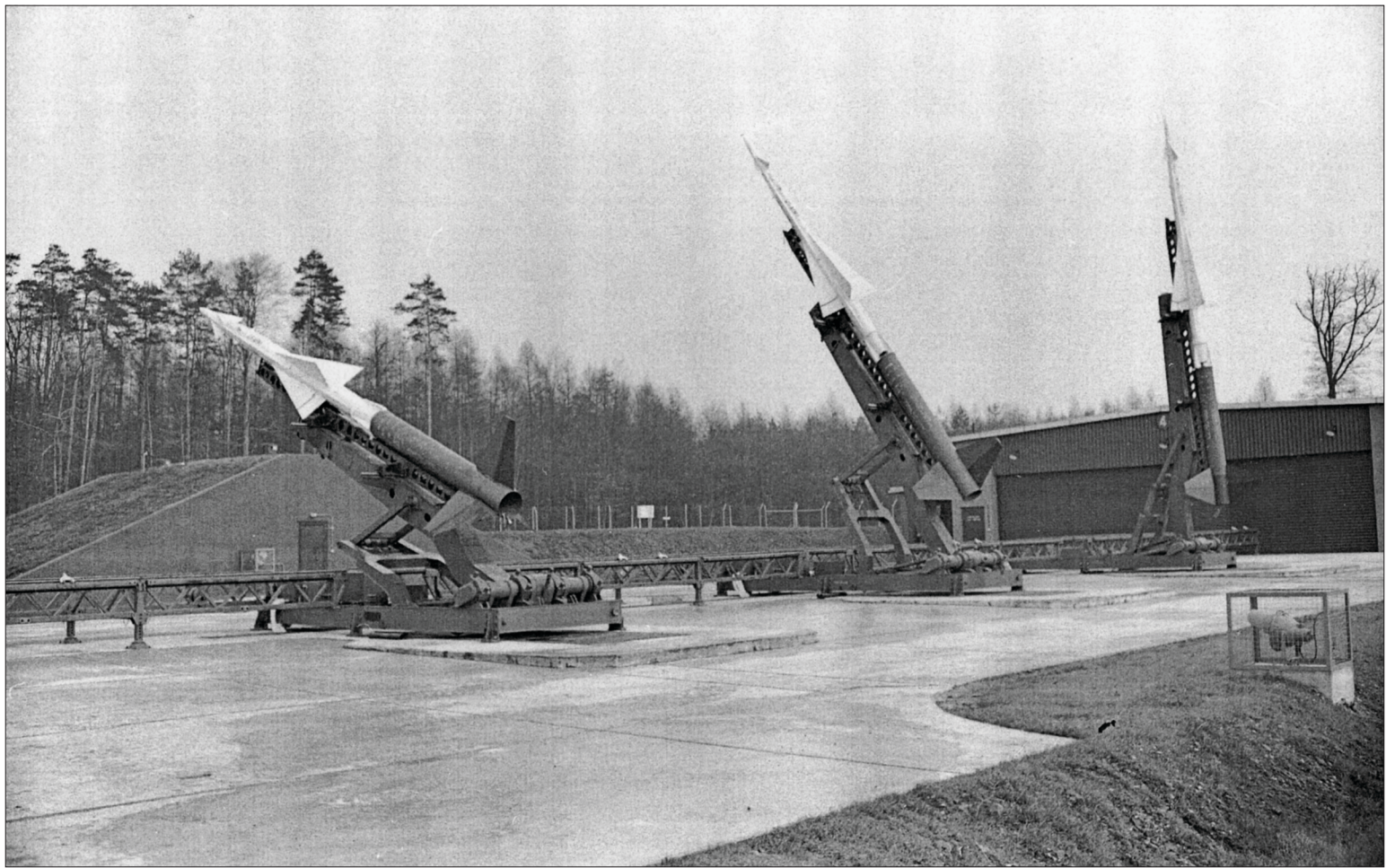
Alpha Section with the crew revetment in the background and the missile storage hanger to the right. The variety of launcher elevations is for show. The far right almost vertical is the correct firing elevation. The lower roof to left of the missile hanger is the section latrine.
