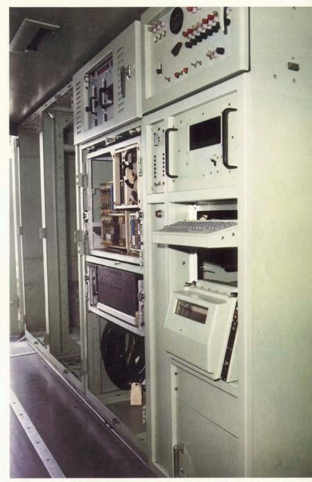
The ICCG includes the Printer/Plotter, Keyboard, Display, Control/Status Panel, Power Supplies, and Power Control Panel. A description of the ICCG equipment follows.
